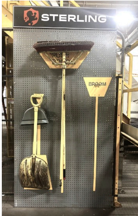
An example of a Lean 5-S implementation at Sterling Structural, Phoenix IL
